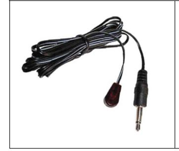
The IR Link OUT is a 3.5mm mono jack socket. The IR signal sensed by the Television is outputted from this socket to an IR emitter (included). This will enable the remote control of external equipment, such as a DVD player from the Television itself.
